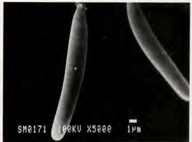
Figure 3. Scanning electron micrograph of isolated nematocysts used for X-ray microanalysis. The white spot represents the site irradiated with an electron beam during the acquisition of spectra. These nematocysts were isolated in DW and incubated in 1 M \text{MgCl}_2 for 10 min.
